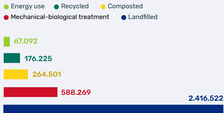
Figure 15. OFMSW use in 2020 (projection from 2017 data) (Eurostat, Annual detailed enterprise statistics for industry, tonnes/year) 9
